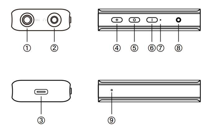
① 4.4mm Headphone Jack ② 3.5mm Headphone Jack ③ Type-C Port ④ Button+ ⑤ Function key ⑥ Button- ⑦ Reset button ⑧ Power button ⑨ Microphone hole
