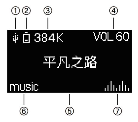
① Connection Method ② Battery Display ③ Decoding Rate ④ Volume ⑤ Lyrics ⑥ Audio Mode ⑦ Dynamic Pickup
