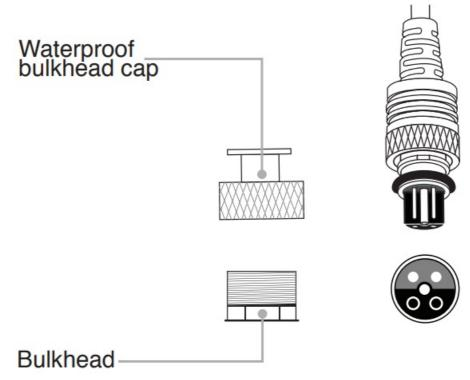
4. Rotate the knurled retaining ring until snug on the housing bulkhead. Do not use pliers or tools to tighten the retaining ring.
