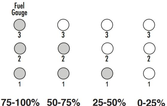
The Fuel Gauge does not indicate remaining battery life when the strobe is in the Off, On, or On w/Lite positions. After briefly displaying the battery level the LEDs will turn off again and the built-in video light will illuminate at the
