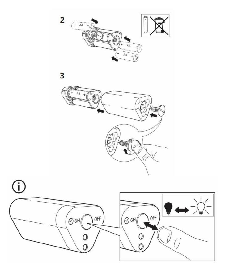
The timer switches the light off automatically after 6 hours, and switches it back on at the same time next day.
