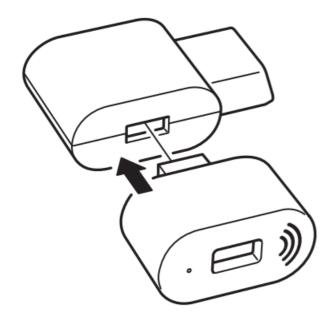
Connect the power supply unit into the wall socket, insert the signal repeater into the free slot.
