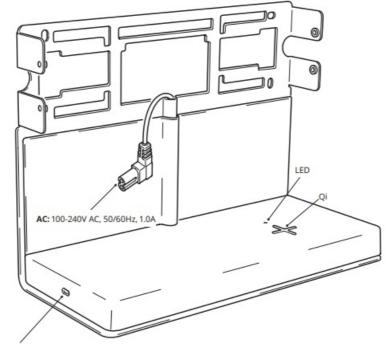
USB-C: 5.0V DC/3.0A 15.0W, 9.0V DC/2.0A 18.0W, 12.0V DC/1.5A 18.0W, 15.0V DC/1.2A 18.0W
