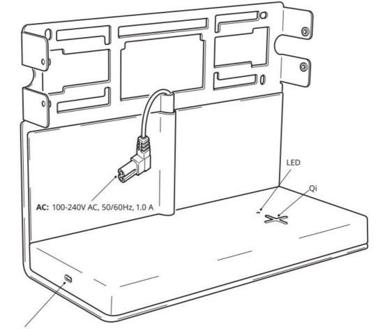
USB-C: 5.0V DC/3.0A 15.0W, 9.0V DC/2.0A 18.0W, 12.0V DC/1.5A 18.0W, 15.0V DC/1.2A 18.0W
