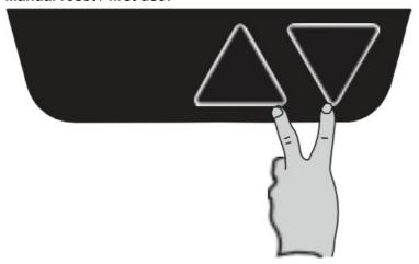
Perform a reset by simultaneously pressing the up and down buttons for at least 8 seconds. Keep holding the buttons and the desk will slowly move to the lowest possible point. Reset is complete when the desk has stopped at the lowest point.
