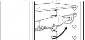
This bottle rack can be tilted to store unsealed bottles. To obtain this result, place front hooks of the rack one level higher than the rear hooks.
