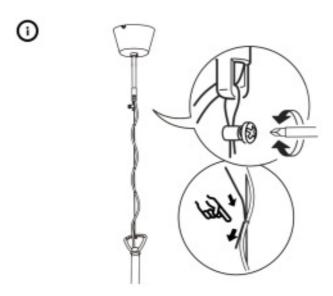
The weight of the lamp must be taken by the suspension wire. When adjusting the cable make sure that it is longer than the wire.
