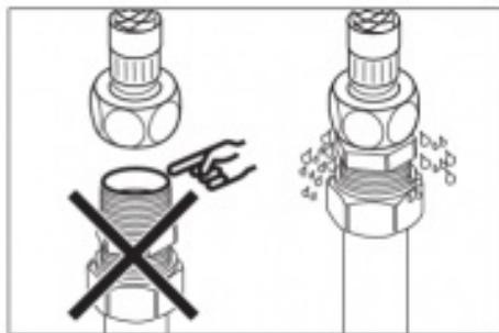
**IMPORTANT!** Do not tighten too hard: this can damage hoses/pipes and washers.
