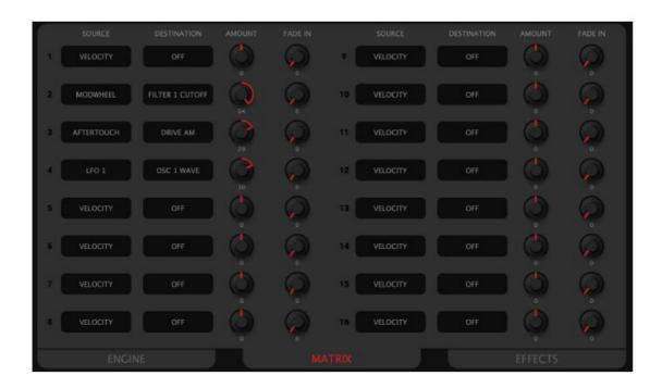
The UNO Synth PRO has a 16-part Modulation Matrix where you can assign a Source to modulate a Destination by a fixed amount. Click the Matrix tab to view and edit the 16 available modulation routes.
