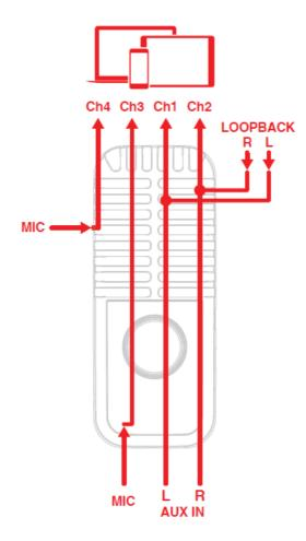
The microphone capsules routing depends on how the polar pattern is set: mono (cardioid, omni and fig.8) or stereo. When the stereo pattern is selected, MIC front capsule is routed to CH 3 and MIC back capsule is routed to CH 4.
