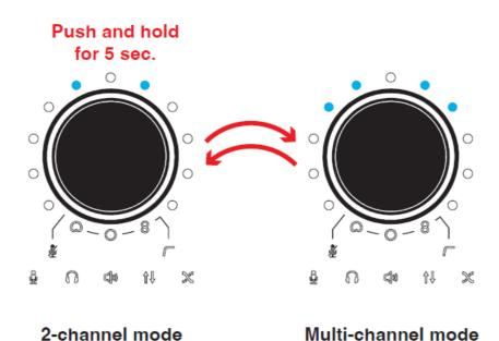
By pushing and holding the knob for 5 seconds the device will enter the operation mode menu. The LED ring will show the current mode selected (2-channel or multichannel). To confirm the operation mode, press the knob and the microphone will restart in the selected mode.
