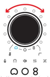
When one of the pattern symbols is blinking blue, you can select the polar patterns by rotating the knob and the
