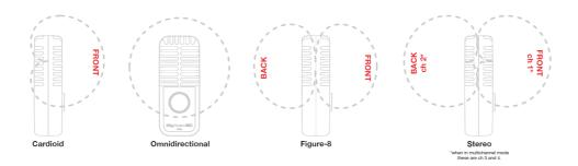
iRig Stream Mic Pro has four different polar patterns to adapt to any recording situation. A polar pattern defines how much of the signal will be picked up by the microphone from different directions.
