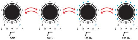
When the HPF symbol is blinking blue, you can select between 4 different high-pass filter settings: OFF - 60 - 100 - 200 Hz. The high-pass filter is useful to get rid of low noises like the rumble of an air conditioner, passing traffic or table vibration. When you move the knob to change the HPF, the LED ring will temporarily show you the selected filter. After 2 seconds the LED ring will return showing the peak level. Press the knob to get back to the Microphone gain control (Section 3.1).
