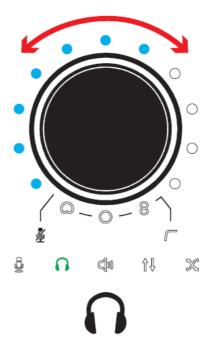
When the headphone symbol is lit green, the knob will control the level of the headphone output and the LED ring will show the peak level of the overall streamed signal.
