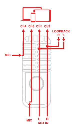
The microphone capsules routing depends on how the polar pattern is set: mono (cardioid, omni and fig.8) or stereo. When the stereo pattern is selected, MIC front capsule is routed to CH 3 and MIC back capsule is routed to CH 4.
