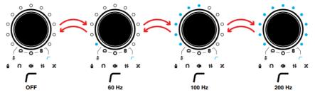
When the HPF symbol is blinking blue, you can select between 4 different high-pass filter settings: OFF - 60 - 100 - 200 Hz.
