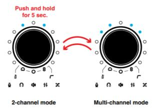
By pushing and holding the knob for 5 seconds the device will enter the operation mode menu. The LED ring will show the current mode selected (2-channel or multichannel).
