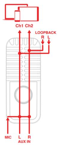
The microphone capsules routing depends on how the polar pattern is set: mono (cardioid, omni and fig.8) or stereo. When the stereo pattern is selected, MIC front capsule is routed to CH 1 and MIC back capsule is routed to CH 2.
