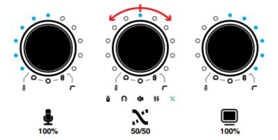
When the monitor mix symbol is lit **green**, you can adjust the mix between the microphone signal and the sound from the connected host in your headphones.
