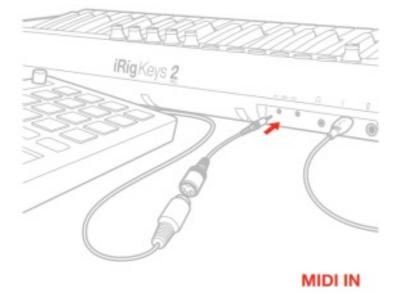
6. To control an external MIDI device, use the included MIDI cable adapter and a standard MIDI cable (not included) to connect the MIDI OUT port of the iRig Keys 2 to the MIDI IN port of the external device.
