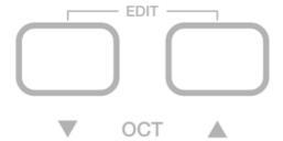
By default, iRig Keys 2 plays notes between C2 and C5. If you need to play notes lower or higher than this range, you can shift the whole keyboard in octaves using the OCT up and down buttons.
