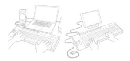
You can start playing as soon as you connect iRig Keys 2 to your iOS device or computer and launch a virtual instrument app or plug-in. Pressing the keys on the iRig Keys 2 keyboard sends MIDI note messages. iRig Keys 2 has a 37-note keyboard that is approximately centered in the middle of a full 88-note piano keyboard.
