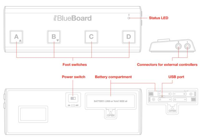
iRig Bluebeard is equipped with four backlit soft-touch pads housed in a sturdy, stage worthy chassis, two TRS jacks for connecting additional controllers like foot switches and expression pedals, and is powered by four standard AAA batteries.
