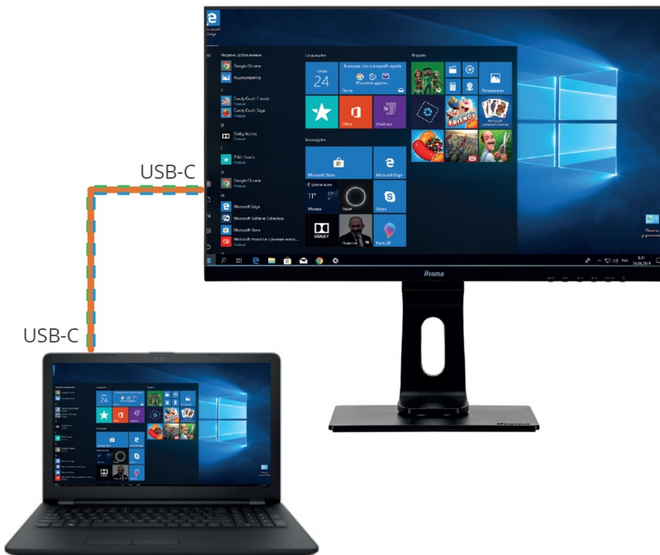
Setup 2 Dual monitor set-up connected to laptop / PC – clone or extension mode
