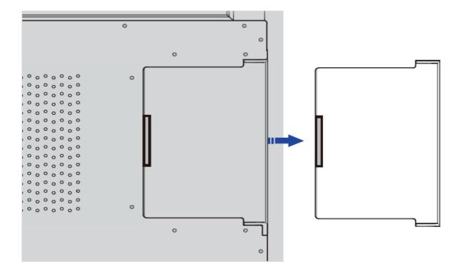
2. Insert OPS PC Module into the panel slot
