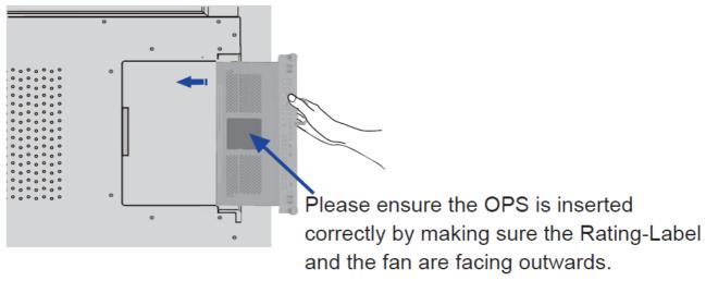
3. Fix the screws or mounting ears and tighten it
