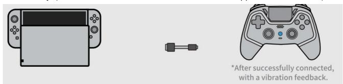
Wired Connection in Handheld Mode: Use the included USB cable connect controller and Switch, The top LED will flash briefly then stay on once connected successfully.
