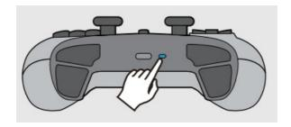
Long press the reset button to reset the controller. After resetting, follow the time connection method to connect the controller.
