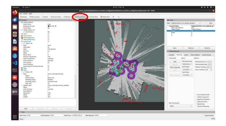
After that, click (and hold) on the map at the estimated position where EduMove is located, then drag in the direction EduMove is oriented, represented by the green arrow:
