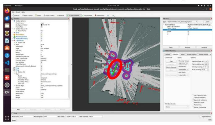
Setting a target position works in the same way. First, select 2D Goal Pose, then click on a point on the map and drag to set the desired target orientation. After this, the planning process within Nav2 begins:
