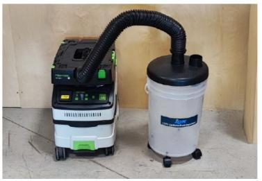
3. Thread the coupler 63 mm on the flexi hose and insert it into the centre hole (hole without elbow). Use another coupler 63 mm or wire clip 63 mm and connect the other hose end to a dust extractor.
