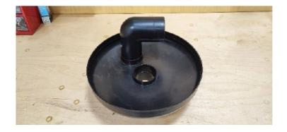
Warning! Make sure the elbow does not face the center hole, otherwise, the separator will work incorrectly.
