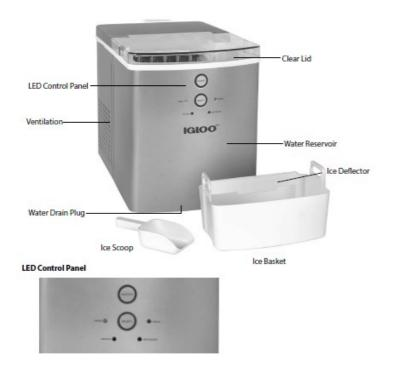
ADD WATER = illuminates when time to add water to Water Reservoir ICE FULL = illuminates when Ice Basket is full S = Small ice cube indicator L = Large ice cube indicator SELECT = press to select size of ice cubes
