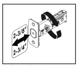
Assemble Keypad Body through latch
