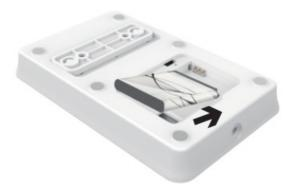
2. If you are using it for the first time, please connect the keypad to the power adapter. The LED indicator will flash while charging until it stays on, which means it is fully charged.
