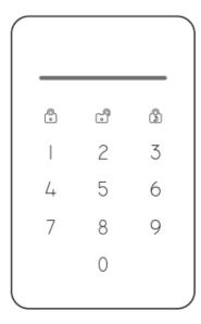
Input the operation code, and press [Arm] [Disarm] or [Home Arm] The status bar would flash once and then change the color as following pattern after command is executed correctly.
