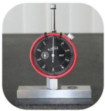
Zero setting when using extension rod and/or flat, needle, or spline point and with a pair of block, and on a flat surface.
