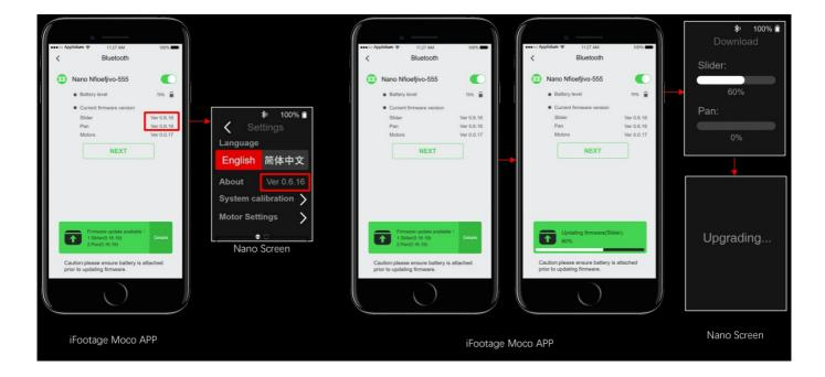
**Step 4**: Turn on the Bluetooth button on the corresponding Nano again, open the iFootage Moco app on your phone. The app will automatically search for the corresponding Nano ID, click the "Upgrade" button again in the app to upgrade the pan axis, wait for the product to automatically restart after the upgrade is complete.
