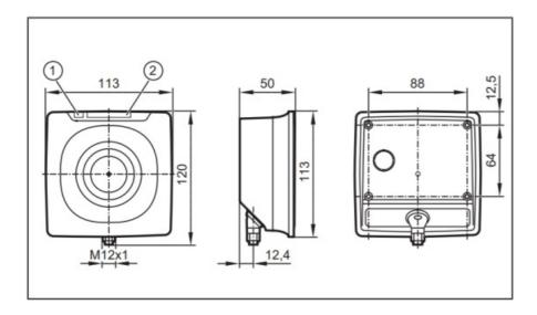
The max. tightening torque of the screws when mounting the device is 0.8 Nm.
