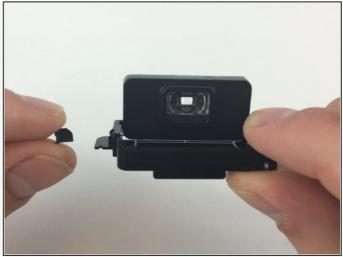
• Once the viewfinder is out, a small black tab should come loose from the viewfinder. Insert this small black tab into the hole on the side of the new viewfinder, with the round side up.
