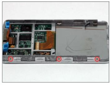
• Remove the three Phillips screws securing the front panel to the metal framework.
