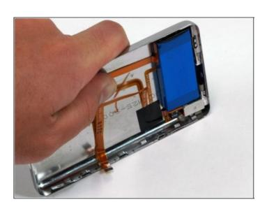
On a clean, hard surface, lay the rear panel on its side. Carefully but firmly push down on it, rolling the entire lip side back into its proper spot.
