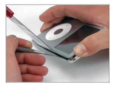
Continue to push up on the front panel with the metal spudger until the metal clip releases.
