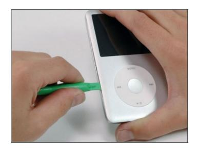
• Insert a plastic opening tool into the seam between the front and back of the iPod.
