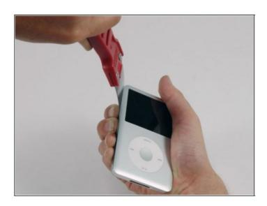
Remove the putty knife from the iPod and reinsert it closer to the corner of the iPod, using the same wiggle method as before.
