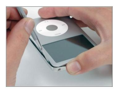
**Step 14:** Gently wiggle the metal spudger down so that it is in the rear panel.
