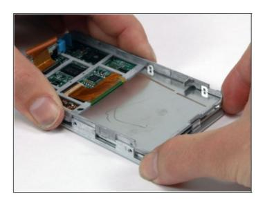
Carefully work around the edges of the iPod to separate the front panel from the gray metal framework.
