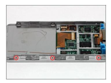
Rotate the iPod 180 degrees and remove the three Phillips screws securing the front panel to the metal framework on the other side.
