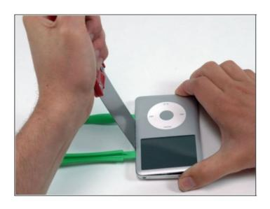
• At an angle, carefully insert a putty knife about 1/8 inch into the seam between the two opening tools.
