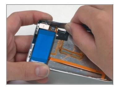
Take the broad, flat side of the metal spudger and push the clip down, taking care not to tear the thin metal rail from the rear panel.
