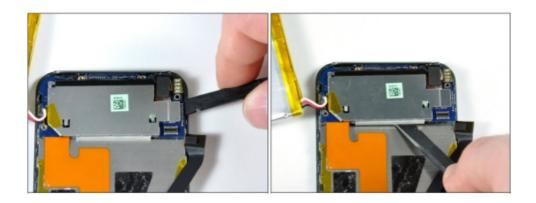
Use the spudger to loosen the logic board from multiple sides. It is held in place by glue and the four screws that were removed in the previous step.
