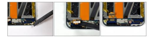
The antenna loop board needs to be pried up (it is glued down). Gently use a plastic opening tool or spudger, to dislodge the antenna loop board. The board is connected to the antenna electronics by a small ribbon cable. This two-board assembly is very frai
