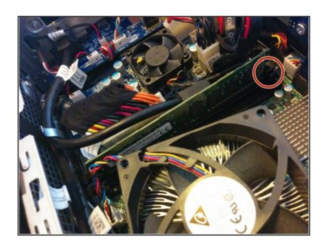
Now, push the white latch (circled in red) DOWN and pull the ram card straight up to a ~45-degree angle. Pull up and out, towards the latch side, and set aside.
