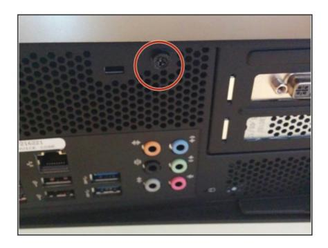
First, turn the computer so you can see the rear panel. Remove the small screw to the right (or above, if the
