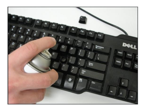
• Clean your keys with compressed air by blowing around the removed key.
