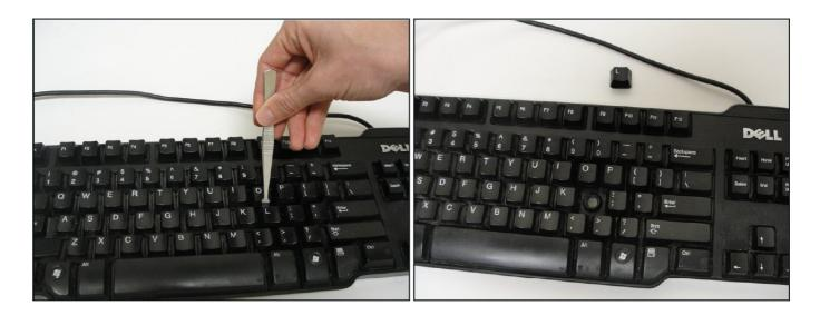
• Wedge the tip of the spudger under the bottom of the key and carefully lift up until the key pops loose.
