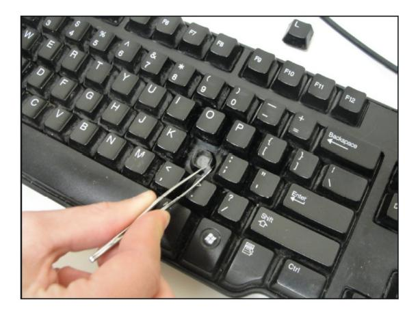
• Use <u>tweezers</u> to remove any contaminants that were preventing the key from being pressed down from the now open hole on your keyboard.
