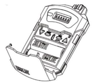
**WARNING!** Do NOT select NiMH (rechargeable) if you are using Lithium or Alkaline batteries; these are primary cells and can be damaged by enabling recharging. Use the NiMH only with NiMH (rechargeable) batteries.
