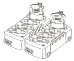
4. Use only rechargeable NiMH batteries and set the battery selector switch in the IFBR1C to NiMH, as shown.
