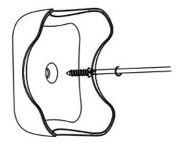
2. **Step two:** P1 serials switch can be adsorbed in switch pedestal, because of the magnet inside.
