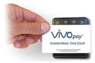
This tests the Kiosk IV's ability to read the Contactless test card. If unsuccessful, there will be no reaction from the reader. If you use a test card and the Kiosk IV antenna is attached to the Kiosk IV Controller, a dummy transaction can be tested. The transaction will not be authorized and will come back with a response but will at least test for end-to-end connectivity.
