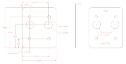
**Note:** Verify the orientation of the Kiosk IV before marking and drilling the holes. The two larger holes should be located towards the top of the mounting location to ensure that the Kiosk IV is oriented correctly with the LEDs at the top.
