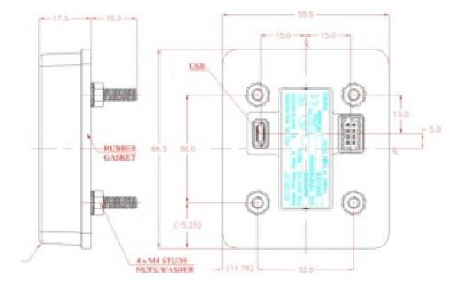
**Note:** The Kiosk IV is post-compatible with Kiosk III dimensions. Posts are 36mm apart in the lengthwise directi on and 32mm apart widthwise. See drawing below.
