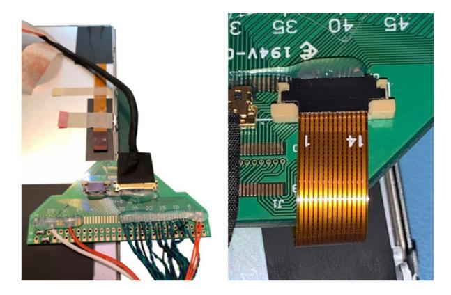
The connections should look like this when the connectors are connected correctly
