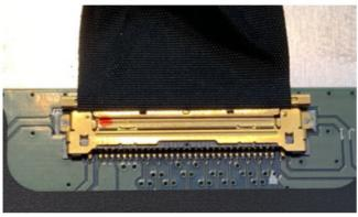
The connection should look like this when the connector is connected correctly.
