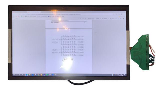
The connections are very fragile and easily torn. It is recommended that all connections are taped and all loose parts are insulated and taped to the rear of the display once the connections have been completed.
