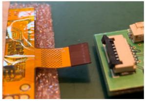
Note the orientation of the FFC and the PCB, it must be connected the correct way round or damage may occur. Push the FFC tail into the connector far enough so that the dark strengthening section is all the way in, and close the flap.
