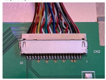
The connection should look like this when the connector is connected correctly.
