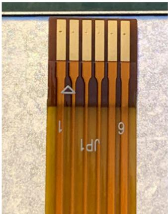
Locate the 6 way 1.0mm connector on the USB cable (Note: Ignore the smaller 0.5mm pitch connector if fitted). Lay the display face down. Lift up the flap on the connector and lay it on top of the FFC tail.
