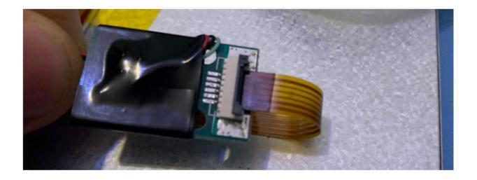
Close the flap to secure the FFC tail
