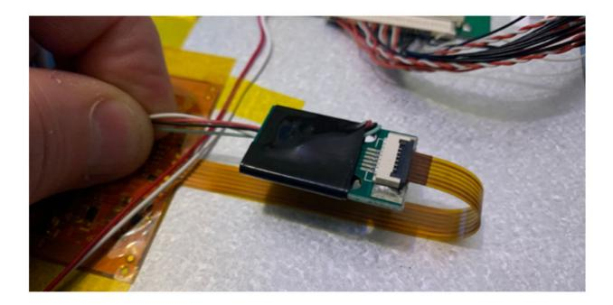
Insert the USB mini connector into the adapter board and connect it to your PC
