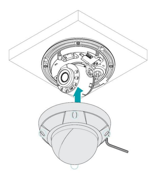
Remove the protective film inside and outside before closing the dome cover.
