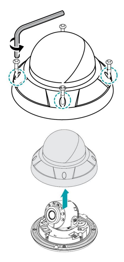
Loosen the screws counterclockwise using the Allen wrench provided with the product.
