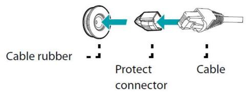
2. Assemble the cable rubber to the bottom cover.
