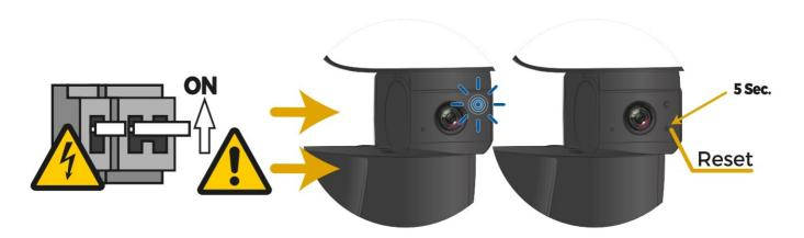
When power in the fuse box is turned back on, the LED indicator will start blinking rapidly. If this is not the case you must reset the device by pressing the Reset button for 5 seconds.
