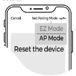
• Press the Reset button for 5 seconds and make sure that the device lights are flashing slowly.
