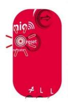
The Red indicator light will be on for 10 seconds to show the reset has been successful.
