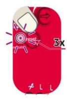
Short press the rest button 3 times. the purple Indictor light will start flashing the will stop flashing and become solid for 10 seconds to show that the device has been successfully.
