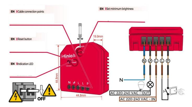
Tum off the power of the specific power group in the fuse box and double check if the existing wall dimmer is really turned off
