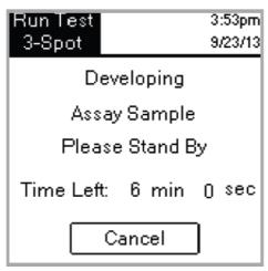
6. After the development time is complete, the SNAPshot DSR Reader takes images of the SNAP test and processes and displays the result.
