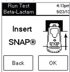
Note: Keep the device in the SNAPshot DSR Reader until the red LED light turns off.
