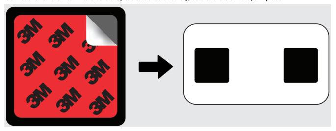
4. Remove the clear plastic from the two square magnets and place the clock on the magnets fixed on the wall. You can adjust the clock's angle as needed.
