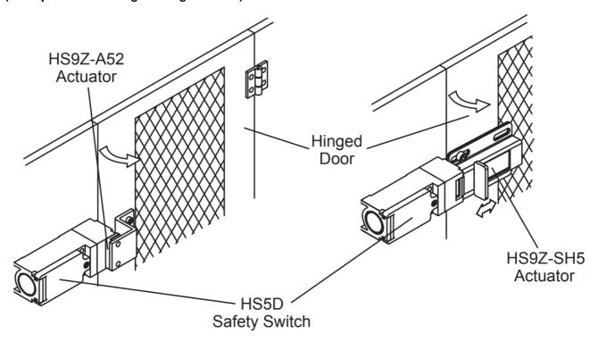
The head of HS5D can be mounted in four directions by removing the four screws on the corners of the HS5D head.
