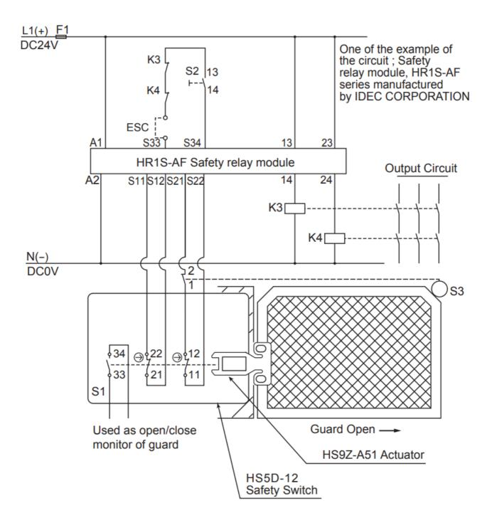
**Note:** Use the monitoring device(Safety relay module) provided the capavility to detect a cross short circuit. The insulation of the cable has to withstand environmental influences. If a control device other than the one shown in the draft is used, the used control device has to be equipped with a cross short circuit monitor.
