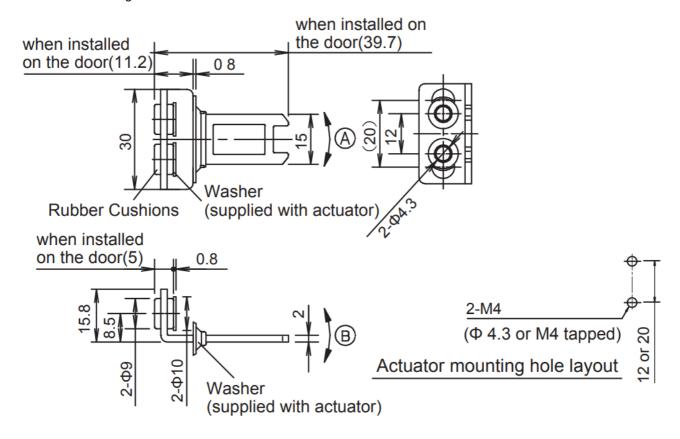
Type: HS9Z-A55 Angle Adjustable (vertical / horizontal) Actuator (horizontal adjustment)
