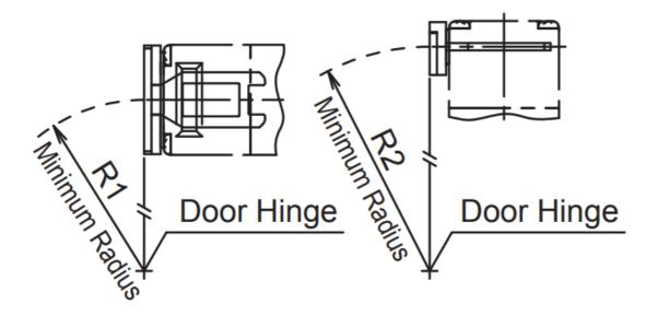
When the center of the hinged door is on the extension line of the contact surface of actuator and safety switch.
