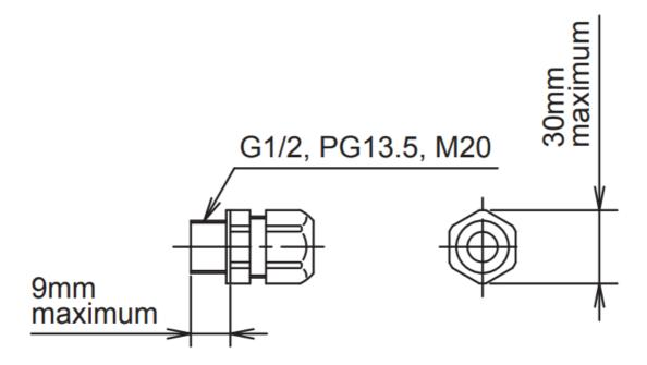
• When using flexible conduit and metal cable gland Applicable Flexible Conduit Example: Type VF-03 (made by Nihon Flex)
