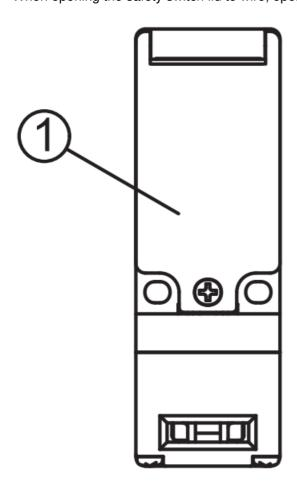
(See the figure on the right.) Never remove other screws, otherwise the safety switch may be damaged.
