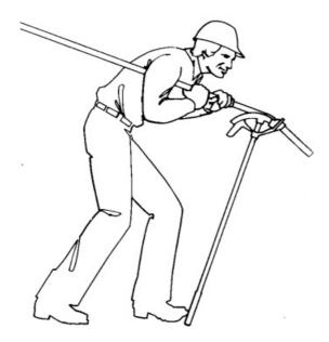
Bend offsets in the air. Remember to keep your body pressure close to the bender.
