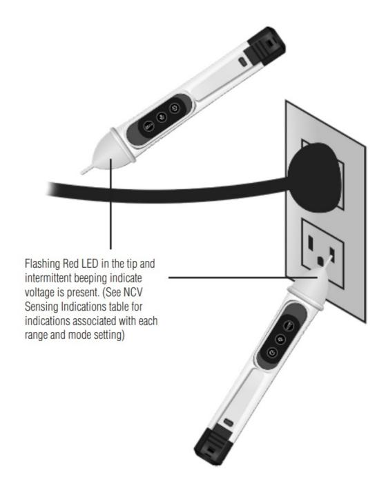
While the NCV is a helpful function, it is ALWAYS RECOMMENDED that the operator verify that any electrical conductor is completely deenergized and that no voltage is present by measuring for voltage AND CONFIRMING THAT NO VOLTAGE IS PRESENT and that all applicable PPE and lock out tag out procedures be followed before attempting any work on ANY electrical distribution system.
