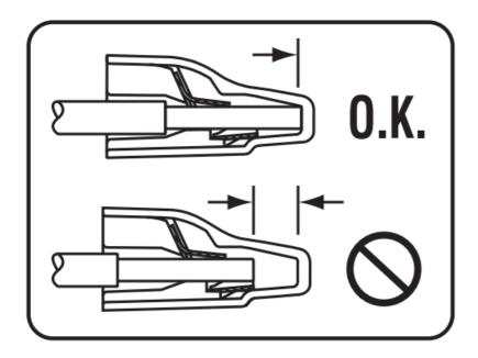
CAUTION: Listed for use with CU or CC. Do Not Use on Aluminum wire. DO NOT RE-USE connector on stranded wire. Consult IDEAL for a complete table of UL Listed and CSA Certified Combinations. For use on insulation types TFN, TFFN, THHN, XHHW, T90 nylon or equivalent. COPPER TO COPPER
