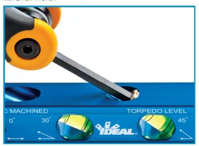
2. Remove O-ring and damaged vial
