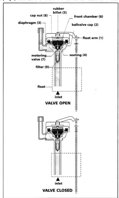
All cistern components must be installed by UK water regulations. If in doubt a suitably qualified professional should be consulted. Ideal Standard UK Ltd., The Bathroom Works. National Avenue. Hull. HUS 4HS
