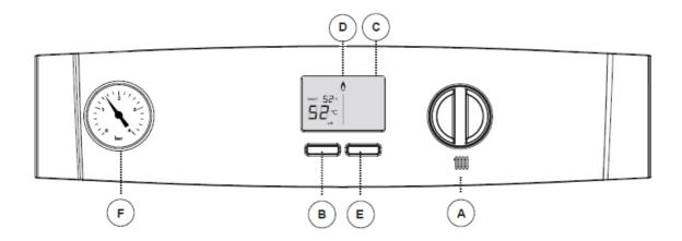
If an L code is shown on the display then the boiler can be restarted by pressing the Restart button (E).
