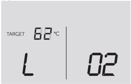
To restart the boiler, press Restart (E). The boiler will repeat the ignition sequence. If the boiler still fails to light consult a Registered Gas Installer.
